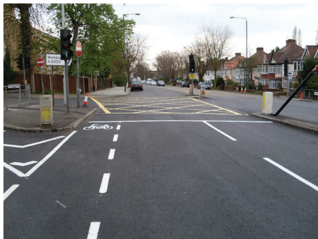
Figure 4. Cycle lane leading to obstruction. This photo shows a cycle lane in a nearside position where there is space on the approach to a junction. The cycle lane does not appear on the other side of the junction and is aligned with the kerb line of the footway. Parking is also permitted across the junction and so cyclists encouraged into a nearside position on the approach would have to move across by at least 4 m to line up with straight-ahead traffic at the point where two lanes of general traffic would merge into one. This transition from secondary to primary position across a junction is referenced as a critical design failure in the cycling level of service assessment (TfL, 2014a). The assessment score is 28 out of 100, meaning it offers a basic level of service. This scheme also has two critical issues – the risk of ‘dooring’ from kerbside activity as cyclists move past the parked cars in a confined space and the choice of putting cyclists into secondary position, that is to say nearside, when approaching a pinch point
